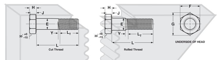
±Length of a cap screw is measured from the underhead bearing surface to the extreme end of the screw.
